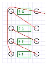
Notice that the path that was "wrapped" around the left pad of R4 is still wrapped even though R4 was moved.
