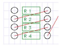
For the next lesson, return to an Equal X and Y spacing of 50 mils. Notice that the resistor pads are now off grid.
