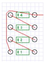
From the tool palette, select the **Move Parts** tool. Use this tool to move R4 up one grid interval like this:
