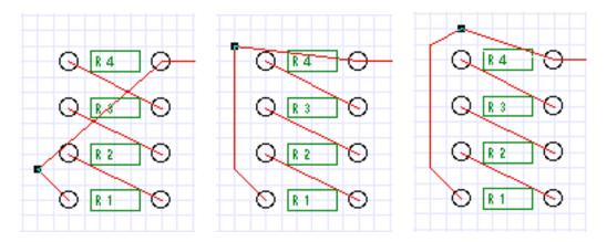
This is like stretching a rubber band around pegs in a peg board. Notice that a small mark appears on the peg nearest the cursor.
