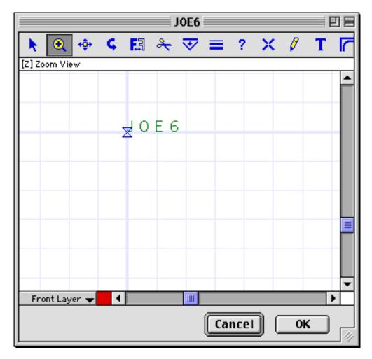
Make sure that the grid spacing is 100 mils by selecting the 100 Mil item in the **Grid** menu.
