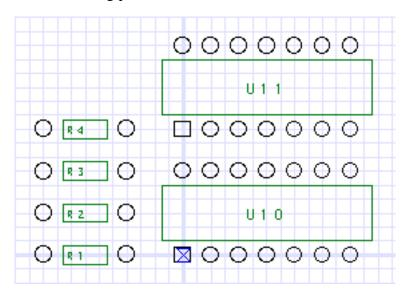
In the previous chapter you used the **Choose/Connect** tool to show what pins should be connected, and to connect paths between these pins. This tool can also make a **Rats Nest**.
