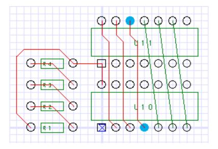
The other bend options are similar. The third option requires paths to extend first in a diagonal direction followed by a horizontal or vertical direction.
