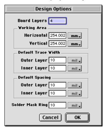
Since we have such a small design, change the Horizontal and Vertical Panel Size to 2.0 inches. Also, change the Default Spacing for both the Outer Layer and the Inner Layer to 15 mils. Notice that the outline of the new panel size is visible in the main view.
