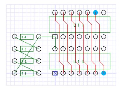
If you click on any of the shorter traces nothing happens since the spacing of the end points of the shorter traces do not match the spacing of the end points of the sampled trace.
