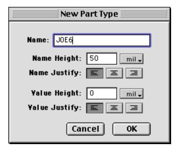
Clicking **OK** allows the **Edit Window** to appear with the origin set in the middle like the picture below. The grid origin becomes the origin of the part type as well. (**Note:** This picture was shrunk a little to allow it to fit in this document.)
