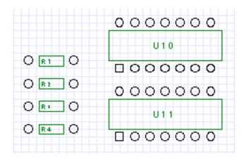
Once the **Deferred Parts** window is empty it can be safely closed. You can now proceed to connect all the pins and route all the paths using the methods learned in the earlier chapters.
