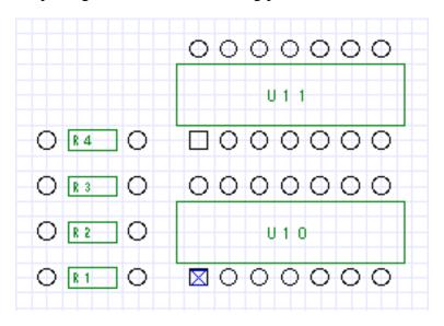
Because this design has a net list, the Osmond program knows what pins should be connected to what other pins. One way for you to see what pins need to be connected is to press the **N** key on the keyboard (**N** is for Next). The view should look like this:
