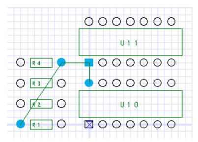
The pins have all been connected by paths on a special layer called the **Rats Nest** layer. Later you will see how to convert these to paths on real layers.
