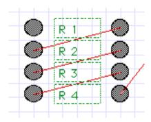
Go back up to the tool palette and select the **Move Parts** tool that you used in the previous lesson. Now use the tool to try to move one of the resistors. You will notice that all the selected resistors now move as a group.
