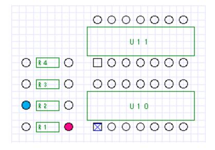
The two pins in color are the two pins that should be connected. Notice that the signal name (\*\*Signal 1\*\*) appears in the text area just below the tool palette.
