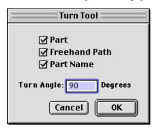
Try changing the 90 Degree turn angle to 30 degrees (for example) and experiment with rotating parts by the smaller angle.
