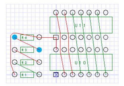
Notice that for straight paths that do not require routing, just clicking on the path is all that is required to place it on the current layer.
