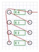
The tool ensures that there is adequate spacing between the path and the pad. To finish routing this path, click and drag the path to the left of the left hand pad of R2 like this:
