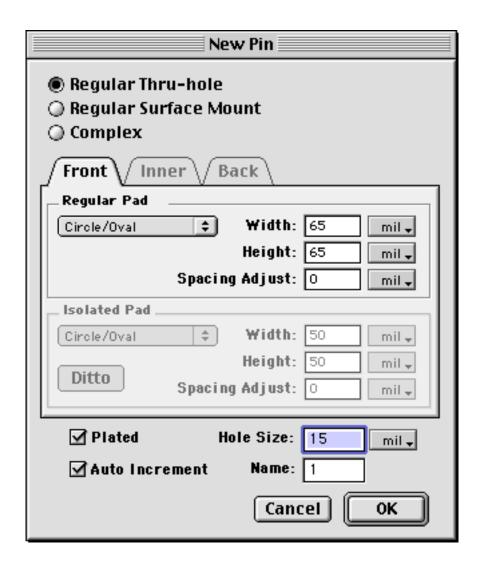
Using the newly configured **New Pin** tool, create a pattern of pins by clicking six times to produce the pattern shown below. If the pattern is not quite right, you can move the individual pins with the **Move** tool.
