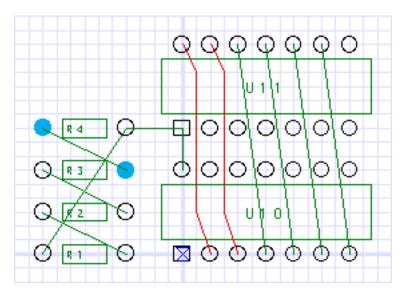
To try out another tool, let us first restore the design to the state in which all signals are connected by **Rats Nest** paths. We can do this by cutting (with the **Cut Path** tool) all paths we have modified, and then by clicking the **Make Rats Nest** menu item in the **Design** menu.
