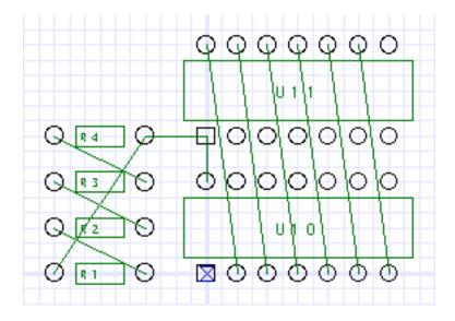
Using one of the normal bend options, route the first long trace between U10 and U11 as shown.
