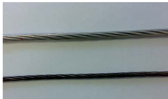
Figure 4 Examples of overhead cables, top 12mm diameter as manufactured, bottom 8mm diameter after weathering
