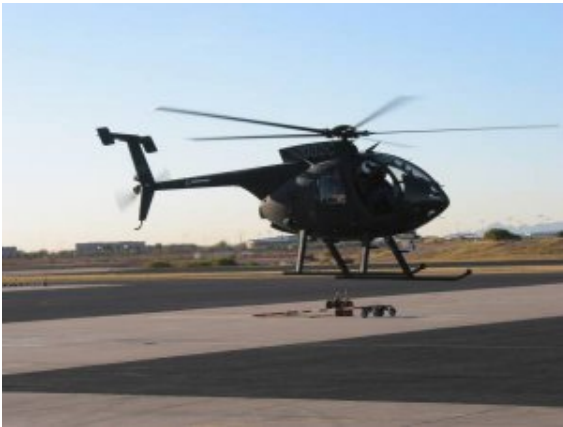
PODS flight test helicopter with chin mounted PODS sensor
